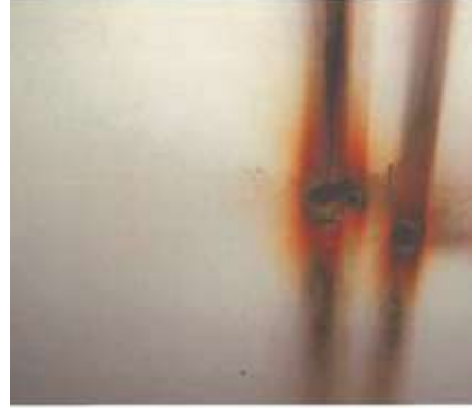
Corrosion on interior shell.
